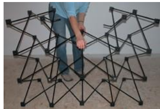
As the frame enlarges, begin pushing the square hubs together.
