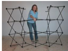
Grab a square hub on the outside, and one on the inside, and push together.
