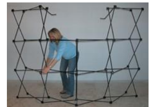
Once the frame is brought to the correct height (6'), connect the plastic hooks to secure it.
